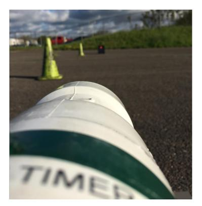
You can sight thru the back of the light to help aim the beam.
